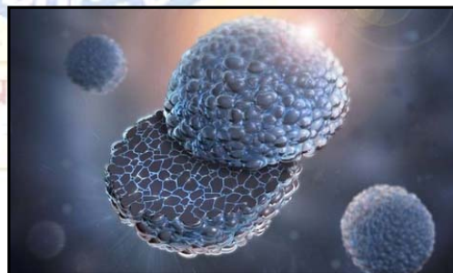
PEDOT is coated on both primary and secondary particles of NMC cathode used in EVs. This coating protects the cathode against reactivity with electrolyte and extends the life of the battery. Credit: Argonne National Laboratory
