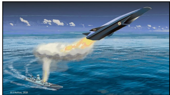
Artist's impression of a hypersonic missile launched from an Indian Navy destroyer. The missile would have a launch booster to get it up to the speed where the scramjet can take over.
