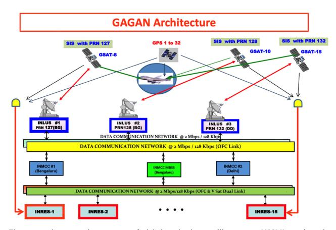
The system improves the accuracy of global navigation satellite system (GNSS) receivers by sending reference signals. The end goal is to develop a navigation system that can be utilised for all stages of flight over Indian airspace and the surrounding areas.
