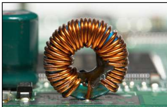
Figure 1: A conventional inductor mounted on a printed circuit board. Inductors have resisted miniaturization until now, but the demonstration of a quantum source of inductance by RIKEN researchers promises to result in much smaller inductors. Credit: GIPHOTOSTOCK / SCIENCE PHOTO LIBRARY
