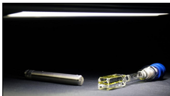
A newly developed molecular system in the glass tube on the right efficiently upconverts visible light even from typical LEDs into ultraviolet light through triplet-triplet annihilation. Developed by researchers at Kyushu University, the system achieves an upconversion efficiency of 20% under high-intensity light, doubling previous records, while also being relatively efficient even under weak light. Credit: Nobuhiro Yanai, Kyushu University
