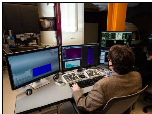
The Radiochemical Processing Laboratory at PNNL is home to a JEOL GrandARM-300F scanning transmission electron microscope, here operated by materials scientist Steven Spurgeon. This specialized facility allows unprecedented atomic-scale characterization of nuclear materials, structural alloys, and functional systems in dynamic conditions. RPL is a Hazard Category II non-reactor nuclear research facility. Credit: Andrea Starr | PNNL
