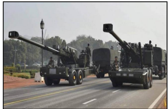
ATAGS consists of dual power system where hydraulics is used for mobility and gun In/out action whereas electrical power is used for Gun laying and Ammunition Handling System.
