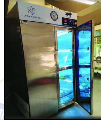
Ultra Swachh can disinfect wide range of materials such as PPE, electronics items.
