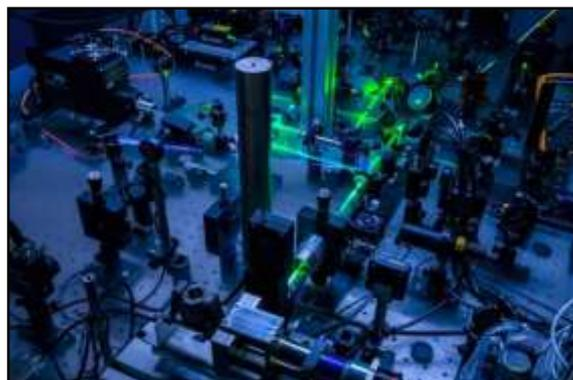
**Amplified frequency-domain thermorefectance setup used to study the existence of second sound in germanium. Two different lasers are focused onto the surface of the samples using a microscope objective. A rather large combination of optical elements allows to control and modify the spot size and shape, as well as the power and harmonic modulation of the lasers. Cold nitrogen gas is used for better visualization of the lasers optical path. Credit: ICMAB, CSIC**
