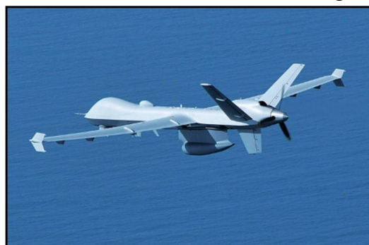
The Sea Guardian UAS manufactured by General Atomics Aeronautical Systems of the US is the naval variant of the Predator B drone which is now known more appropriately by the name MQ-9 Reaper.
