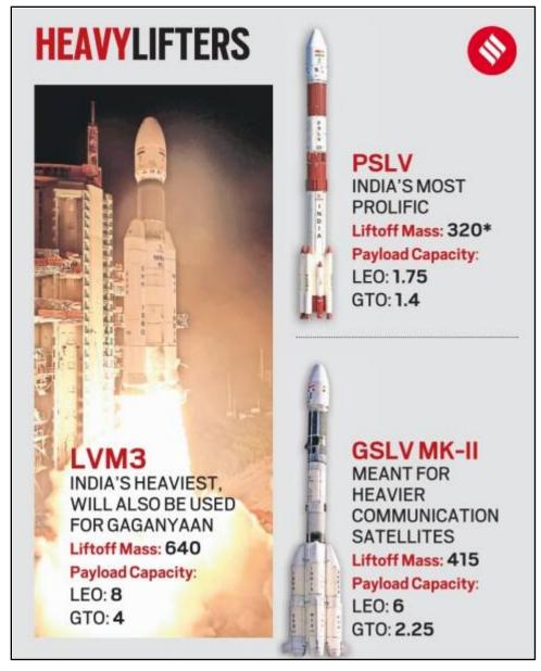
The PSLV has been the most commonly used, having carried as many as 53 successful missions since 1993. Only two flights of PSLV have failed.
