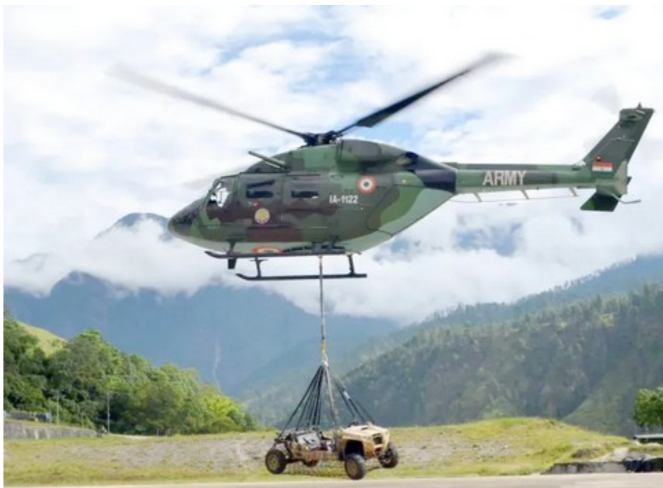
An Advanced Light Helicopter carries an ATV in an underslung configuration to enhance operational and logistic stamina in forward areas.
