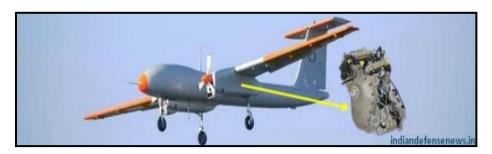
TAPAS BH-201 is currently flying with an imported AUSTRO AE300 Diesel-Kerosene Engine
