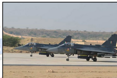
This is an indigenous four and a half-generation tailless compound delta-wing aircraft. (Photo source: HAL)
