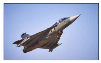
The Hindustan Aeronautics Limited (HAL) Tejas Mark 2 is a single-engine multirole fighter designed by Aeronautical Development Agency (ADA) and HAL. The plane has tailless compound delta-wing configuration with high manoeuvrability.
