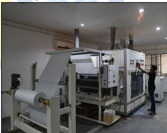
A textile engineer at Ahmedabad Textile Industry's Research Association (ATIRA) monitors an electrospinning machine, which is used to make filters for N99 masks for the Defence Research and Development Organisation (DRDO), during a government-imposed nationwide lockdown as a preventive measure against the spread of the COVID-19 coronavirus in Ahmedabad on April 17, 2020. (Photo by SAM PANTHAKY/AFP via Getty Images)
