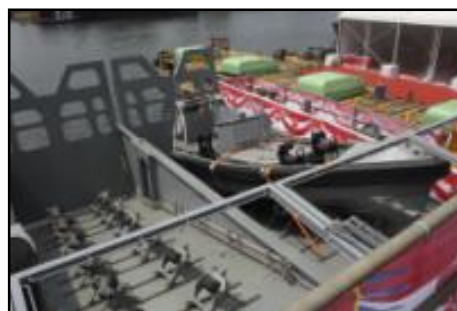
A view of the automated launch-and-recovery system installed on an Independence-class vessel. (Janes/Ridzwan Rahmat)
