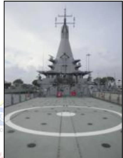
The flight deck of RSS Sovereignty , which has been designed to embark rotary-wing UAVs but not helicopters. (Janes/Ridzwan Rahmat)
