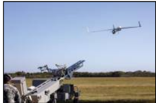
822X Squadron launching a ScanEagle via a pneumatic launcher. (Commonwealth of Australia)
