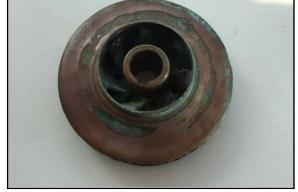
energy from the motor to the fluid being pumped by accelerating the fluid outwards from the center of rotation. On ships it is used to import seawater to sections of the ship for regular water needs. Impellers often come in different shapes and sizes according to the amount of liquid to be pumped. They are required to rotate at high speeds for long periods of time.
