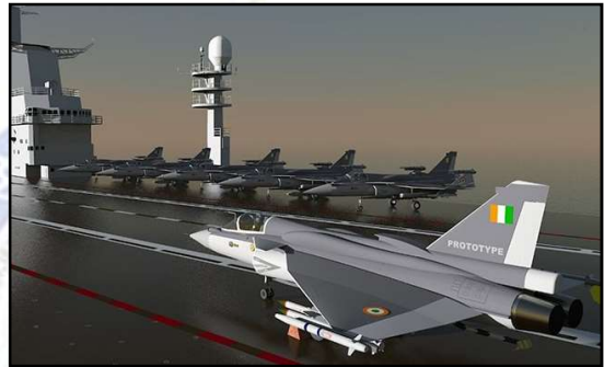
The twin-engine deck-based fighter is meant to operate on India's aircraft carriers.
