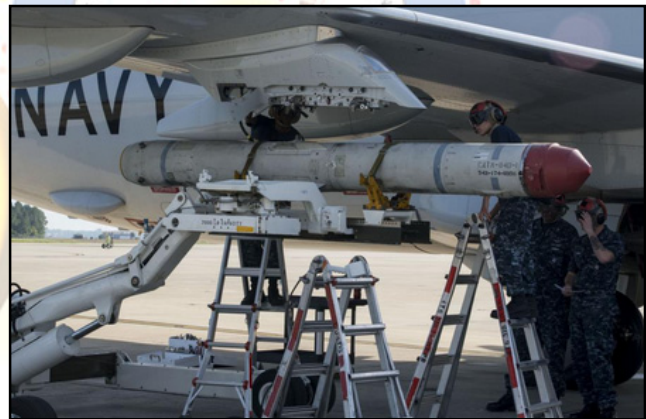
AGM-84K SLAM-ER missile on a P-8A Poseidon at Naval Air Station Jacksonville in Florida
