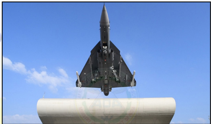
The naval Tejas fighter taking off from the ski-jump with Derby's (mounted on the inner-wing hardpoints) and R-73s (painted white, on outer-wing hardpoints) | Twitter handle of DRDO
