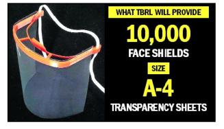
The face shields are light weight and can be worn full day with comfort. Commonly available A-4 size transparency sheets used in overhead projectors are being used as visors while the holding frame is manufactured through Fused Deposition Modeling (FDM), commonly known as 3-D printing. Polylactic Acid filament, a biodegradable thermoplastic derived from renewable resources such as corn starch or sugarcane, was used for 3-D printing.
