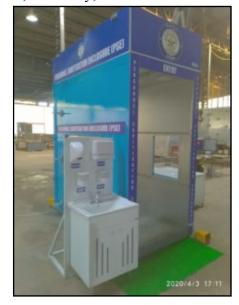
sodium chloride for disinfecting. The mist spray is calibrated to operate for 25 seconds and stops automatically thereafter, indicating completion of the operation. Approximately 650 personnel can pass through the chamber for disinfection until a refill is required. The system has a see-through glass panel as sidewalls for monitoring and is fitted with lights for illumination during night time operations.
