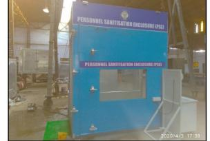
placed tanks with a total of 700 liters capacity. Approximately 650 personnel can pass through the chamber for disinfection until the refill is required. A separate operator cabin is provided to monitor overall operations.
