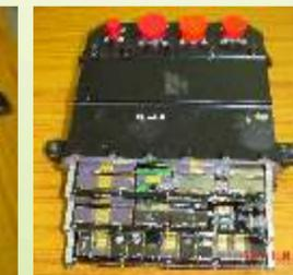
banks, MIL-STD-1553B bus module supporting two channels of BC/RT/MT are some of the special features of the computer. Intelligent analog and digital I/O modules based on Intel 87C 196 micro-controller comprising ADC and DAC channels control the interface functions. The computer has been successfully flight-tested.
