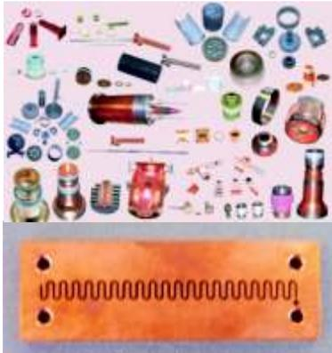
Folded waveguide SWS, and components and assemblies (top)
