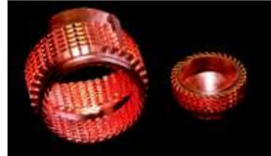
Septums used in the SWS of CC-SWS and collector parts
