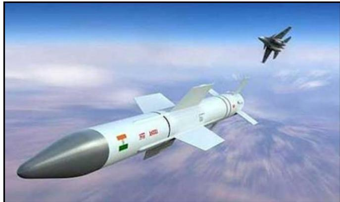
The Astra is designed to carry 15 kg high explosive prefragmented warhead, which is activated by a Radio Proximity Fuse. The missile has good Electronic Counter-Countermeasure (ECCM) to enable unconstrained operation in an Electronic Countermeasure (ECM) environment. The Astra Mark 1, which successfully completed the trials recently, has a maximum head-on launch range of 100 km, a speed of 4.5 Mach and is cleared for launch up to an altitude of 20 km (66,000 ft).
