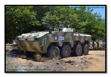
vehicle called WhAP (Wheeled Amphibious Platform) developed jointly by the DRDO's Vehicle Research and Development Establishment and the Indian Company TATA Motors. The Whap is fitted with a two-man **BMP-2** turret, a Soviet-made Infantry Fighting Vehicle.
