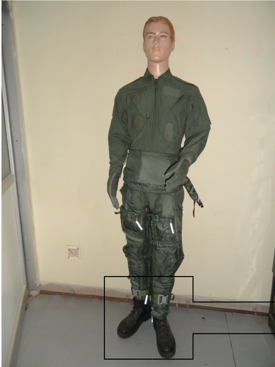
GARTERS LEG RESTRAINT – HAWK WORN ON THE LOWER LEG PORTION OVER THE ANTI G SUIT
