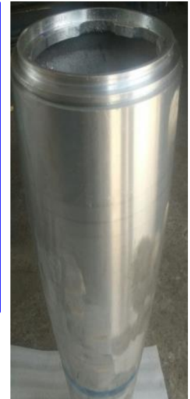
Al-Alloy Shell Finished Component for Underwater Application
