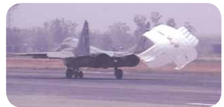
Unicross brake parachute for MiG-29
