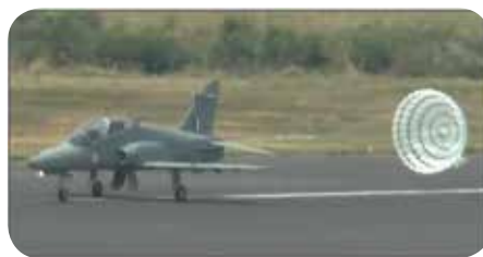
Ring slot brake parachute for hawk (AJT)
