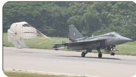
Unicross LCA brake parachute
