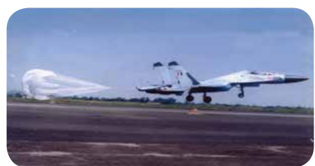
Unicross twin canopy brake parachute for SU-30
