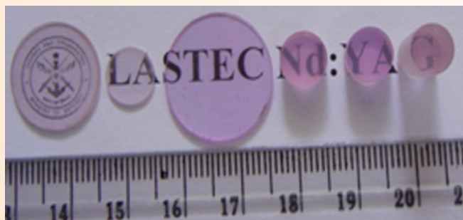
Nd:YAG Polycrystalline Ceramic
