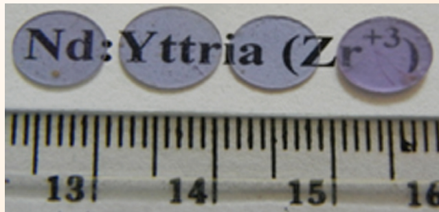
Nd:Yttria Polycrystalline Ceramic
