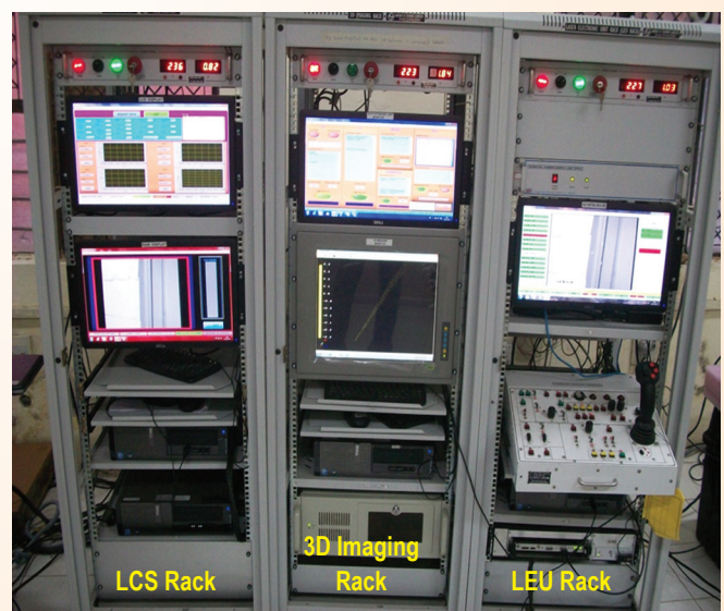
LACSMI Electronic System consisting of LCS and 3D Imaging Unit
