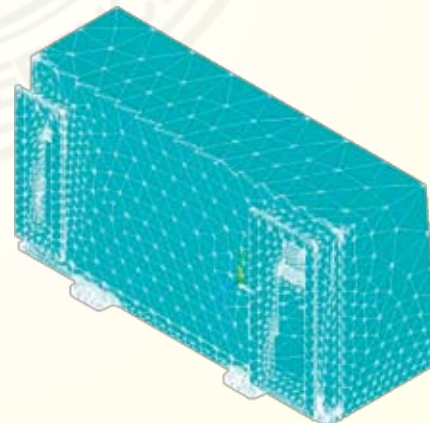
Displacement contours under vibration (MCS-3547)
