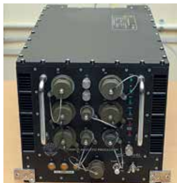
Conduction Cooled T4241 SBCs in Signal Processing ATR
