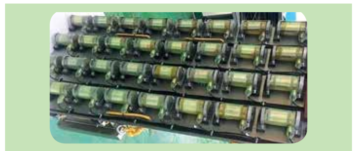
32 Mandrel Hydrophones Arrayed in a Planar Form
