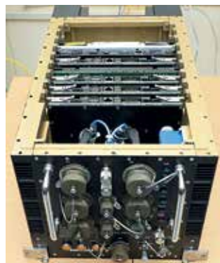
Conduction Cooled T4241 SBCs in Signal Processing ATR
