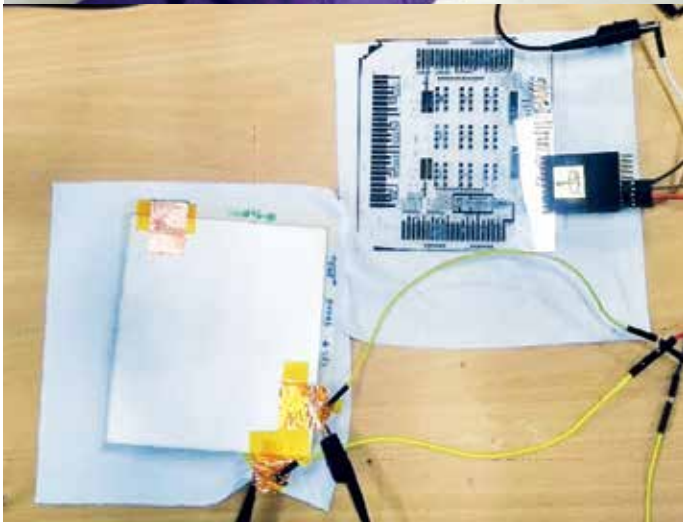
(a) IGZO TFT Amplifiers on PEN (b) Measurement of Amplifier Response with PVDF Sensor
