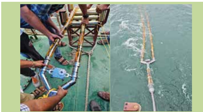
Twin Array During Deployment and Towing on-board MV Kurathi
