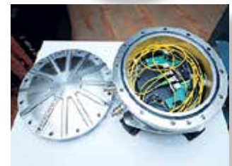
32-channel Data Acquisition system
