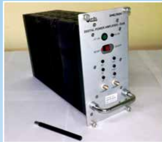
PWM based Full Bridge 8000 Wrms PA
