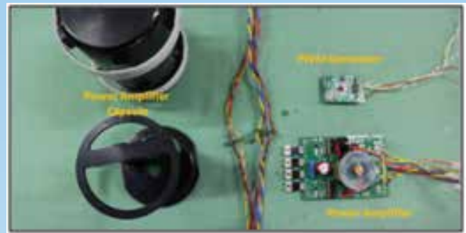
Power Amplifier Capsule and PCBs used in HPA
