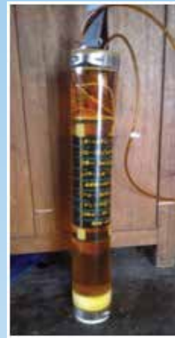
A Module of nine Flexural Disc Projectors inside a Test Fixture
