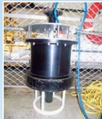
Cylindrical Piezocomposite Transducers (Projector and Sensor Arrays) Assembled with the Electronic Unit
