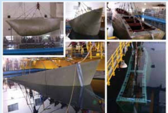
Sonar Dome being Deployed in the Acoustic Tank at NPOL
