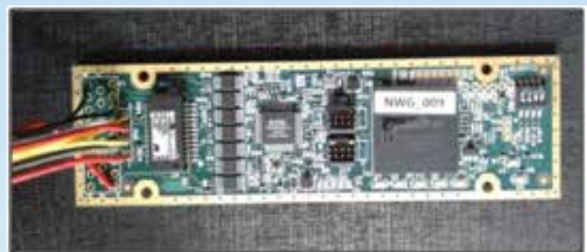
Signal Distribution PCB for HPA
