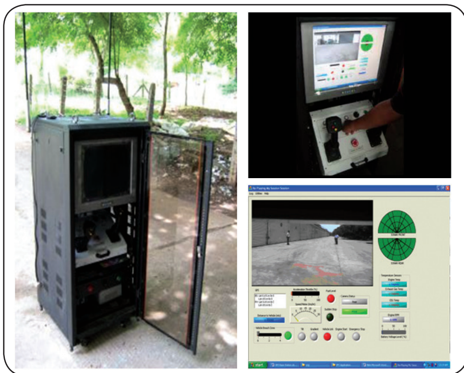
Base station for Tele-operated ATV
