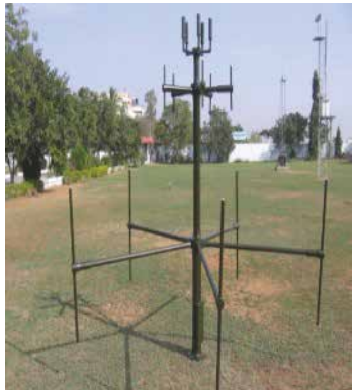
DF Antenna sub system for COMINT
