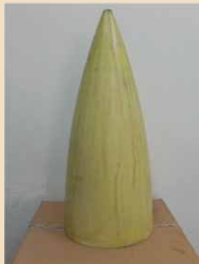
Prototype of Scale Model of Multilayer Radome
