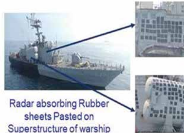
ISAR Imaging Modification of Warship Using Radar Rubber Absorbing Sheet
