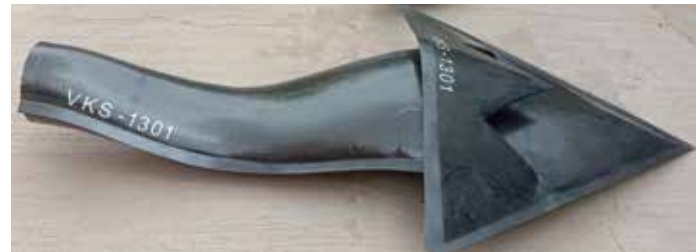
Model Duct Fabricated with Magnetic Flakes
