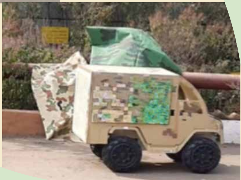
Visible Adaptive Add-on for AFV to Adapt to Changes in Colour and Patterns
