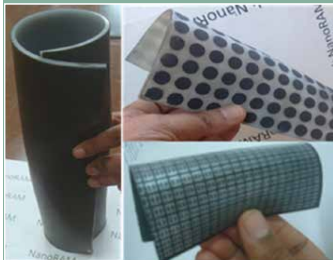
Flexible Rubber-based Absorber
