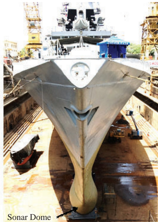
GFRP SONAR dome; as manufactured and as fitted on INS Kolkata
