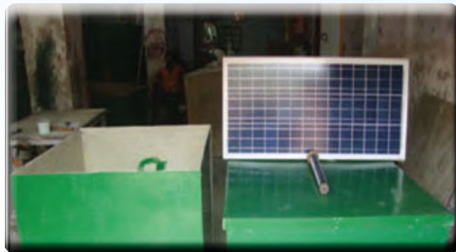
FRP Biodigester for Low Temperature Areas (Leh)-Single Family
