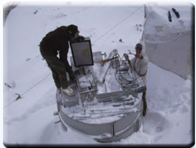
Temperature Controlled Modular Biodigester for Glaciers
