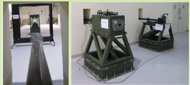
Indoor Experimental Set-up of Propellant Guns at Ballistic Test Facility
