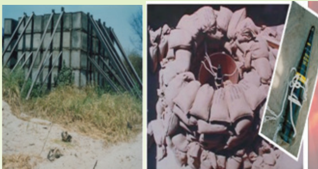
Sand Pit Fragmentation Chamber
