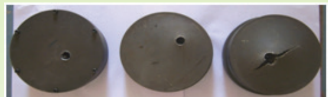
Impact Sensitivity Test on Explosives (Fragment Impact Test)
