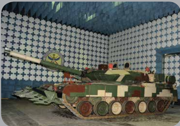
Arjun MBT Mk-II inside EMI/EMC test facility
