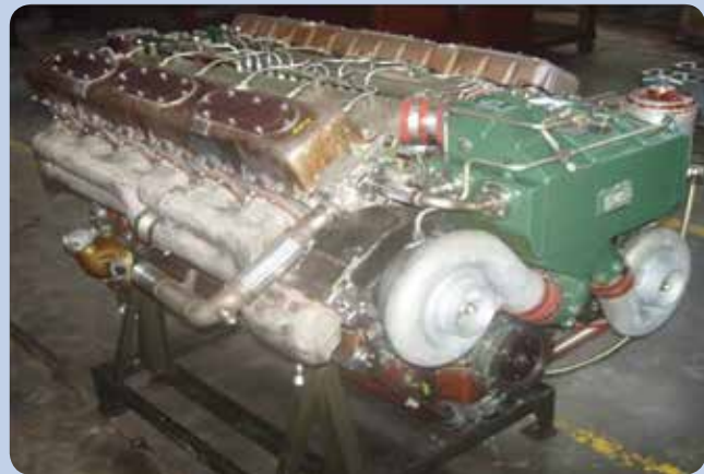
T-72 Engine uprated by CVRDE
