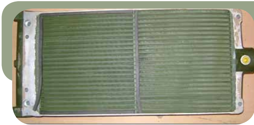
Side Radiator-Arjun MBT
