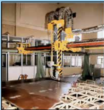
Manipulator for NDT of LCA Components, Hot-slug Handling and Eddy-current Testing of Steam Generator Tubes
