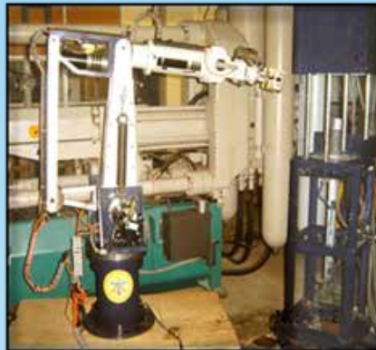
Manipulator for NDT of LCA Components, Hot-slug Handling and Eddy-current Testing of Steam Generator Tubes
