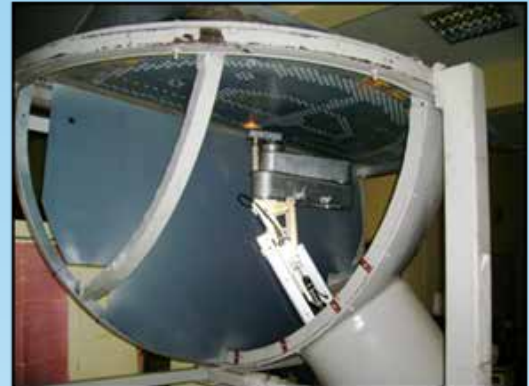
Manipulator for NDT of LCA Components, Hot-slug Handling and Eddy-current Testing of Steam Generator Tubes
