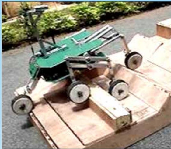
Wheeled Robot with Passive Suspension
