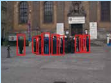
Human Detection in Optical Images (Red rectangle marks the detection of the algorithm)
