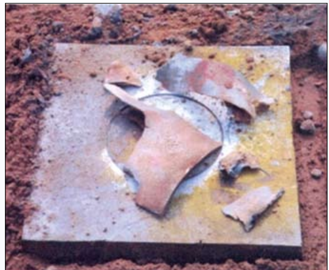
Witness Plate & Fragments of Pinaka Motor Casing
