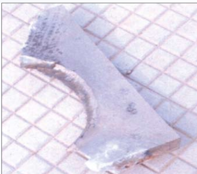
Sheared Piece of Witness Plate by NEPE Propellant
