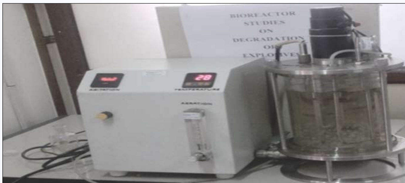
Lab-scale Bioreactor used for Degradation Evaluation of TNT and DNT
