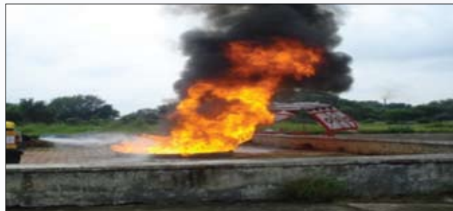
Flammable Liquid Pool Fire Suppression
