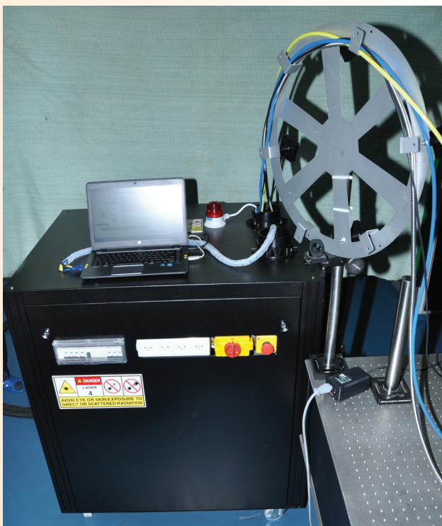
1 kW Single Mode Fiber Laser
