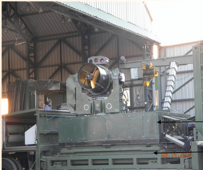
Dual Axis Stabilised Gimbal Assembly Integrated on BDV (ADITYA)
