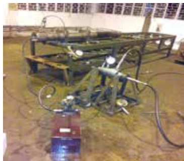
Pressure Testing of Recoil System
