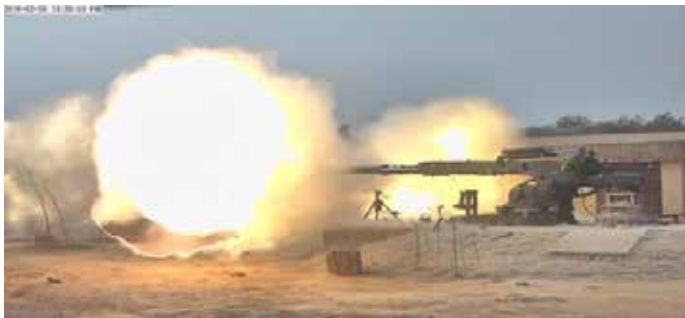
First Firing of ATAGS Barrel at P 2 Pressure at PXE, Balasore
