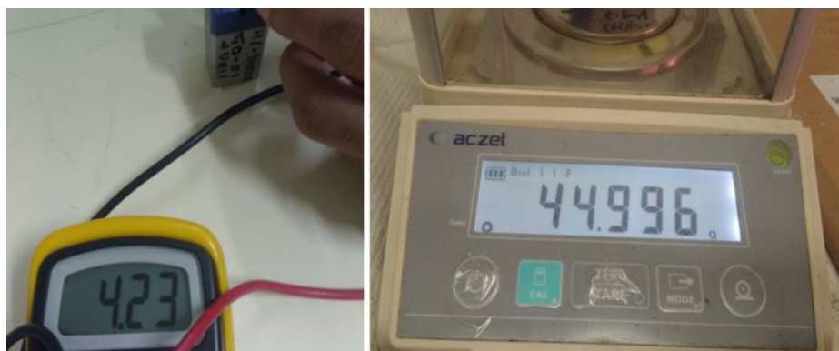
BPC/rGO batteries of 4.2 V and weighing 45 g
