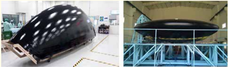
Realized composite radome & integration with metallic structure
