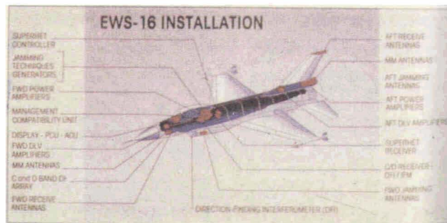
Fig. 5.4 Layout of EWS-16 Electronic Warfare system fitted on F-16 fighters
