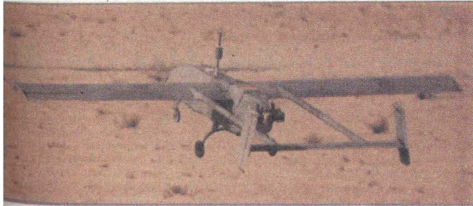
Fig. 5.14 Pioneer, the UAV used in Gulf war for bomb damage assessment and other work
