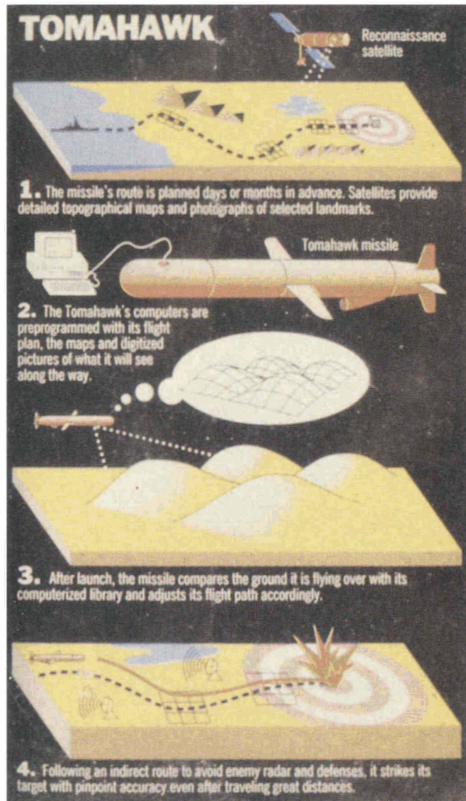
Fig. 5.8(a) Four phases of pre- and post-launch activities of Tomahawk cruise missile
