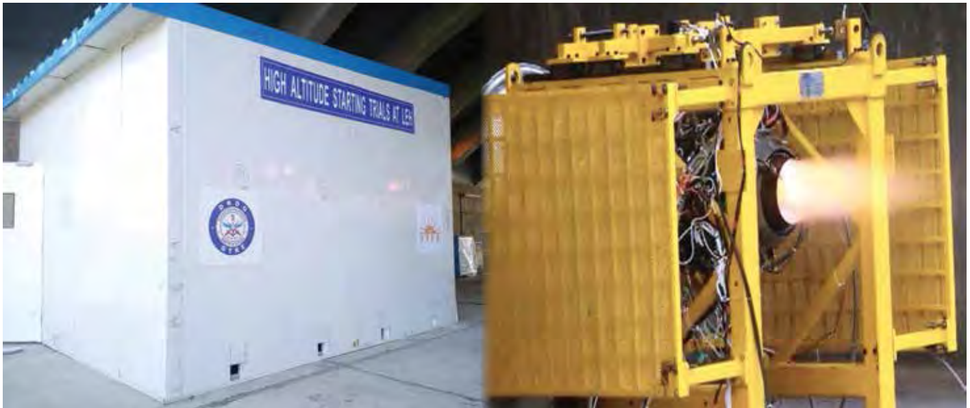
High Altitude starting trials of small turbo fan at Leh.
