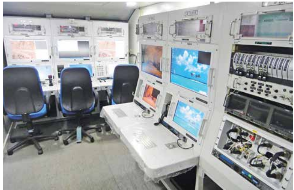
Tapas-Ground Control Station
